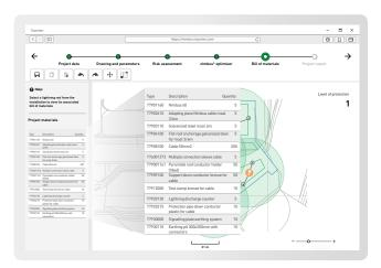
The software generates the overall bill of materials (lightning rods and accessories) required for the protection of the comprehensive facility, in addition to a bill of materials for each lightning rod.
